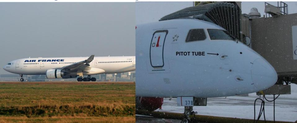
"At 02:10:05 UTC the autopilot disengaged because the blocked pitot tubes were no longer providing valid airspeed information, and the aircraft transitioned from normal law to alternate law 2. The engines' auto-thrust systems disengaged three seconds later. Without the auto-pilot, the aircraft started to roll to the right due to turbulence, and the pilot reacted by deflecting his side-stick to the left."
